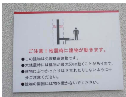
(a) Overview of the building (b) Sign board to warn about seismic gap
