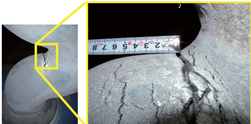
Photo 9.2-17 Lead damper and cracks on the surface
