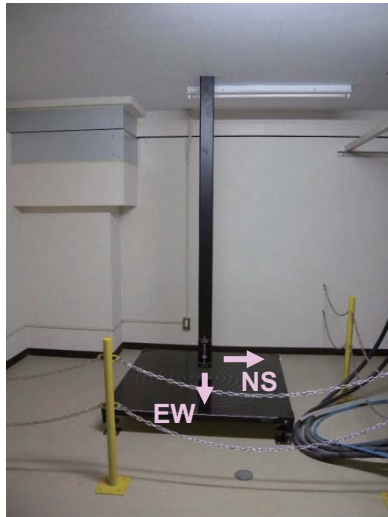
Photo 9.2-3 Scratch board installed on the SI floor
