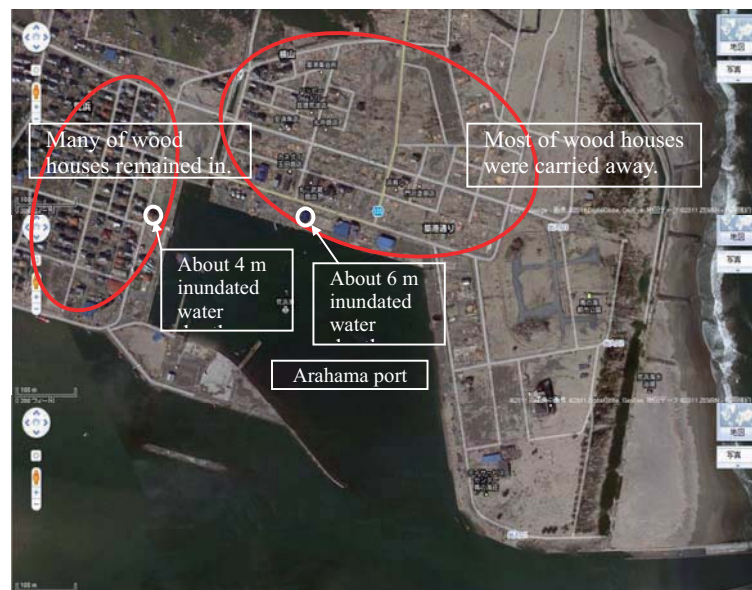
Fig. 7.4-3. Aerial photograph and the water depth estimated in Arahama, Watari town.
