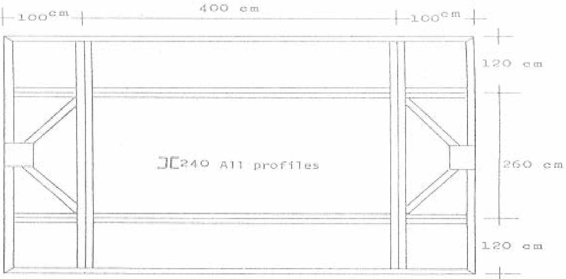
Figure-3 Plan View of the Steel Frame of the Table
