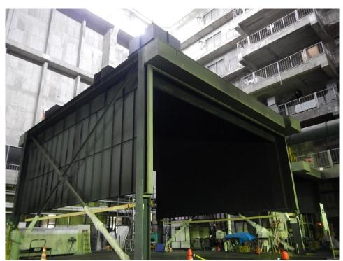
Fire test hall with smoke exhaust hood used for measuring heat, smoke and gas generated from combustion. (7 story smoke control test tower is seen at right rear.)
