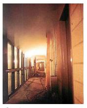
Smoke movement test at corridor
