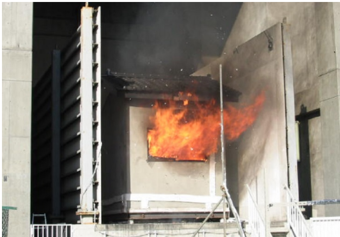
Ejected flame from an opening under wind
