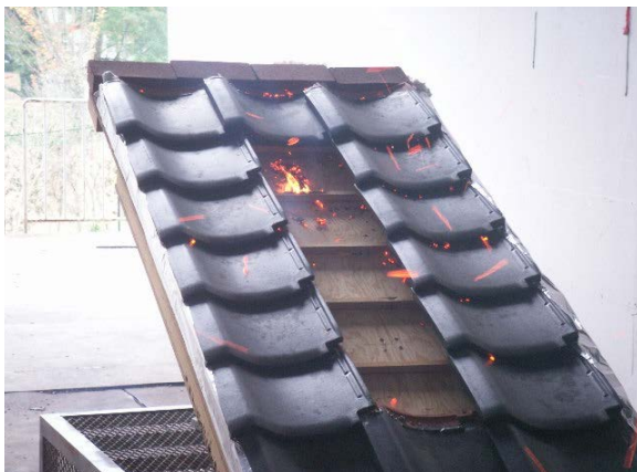
Roof ignition due to firebrands
