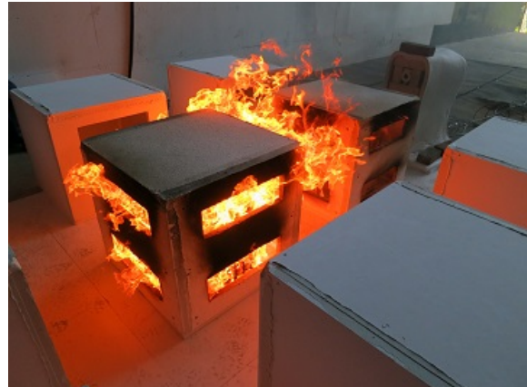
Fire spread between model buildings
