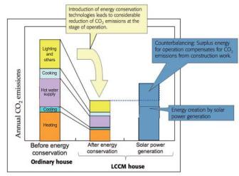
Figure 6: Energy Balance of the LCCM House
