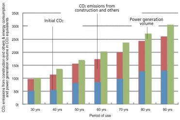
Figure 8: Trend in CO<sub>2</sub> Emissions and Power Generation Volume (Under the condition with the use of a solar thermal hot water system with natural refrigerant and with the unit CO<sub>2</sub> emissions of 0.418 kg-CO<sub>2</sub>/kWh on average for all power sources)
