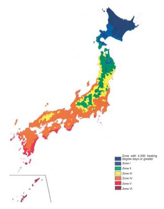
Figure 4: Zone Classification under the Act on the Rational Use of Energy
