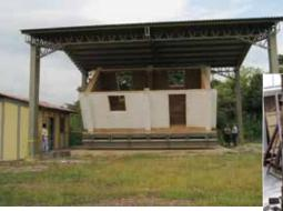
An improved adobe structure was successfully tested on the incline platform built at the University of El Salvador.
