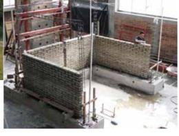
A framework masonry test structure using the soil-cement method under construction at Central American University
